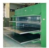
FURNACE WITH SUPERIMPOSED VENTILATED CHAMBERS
